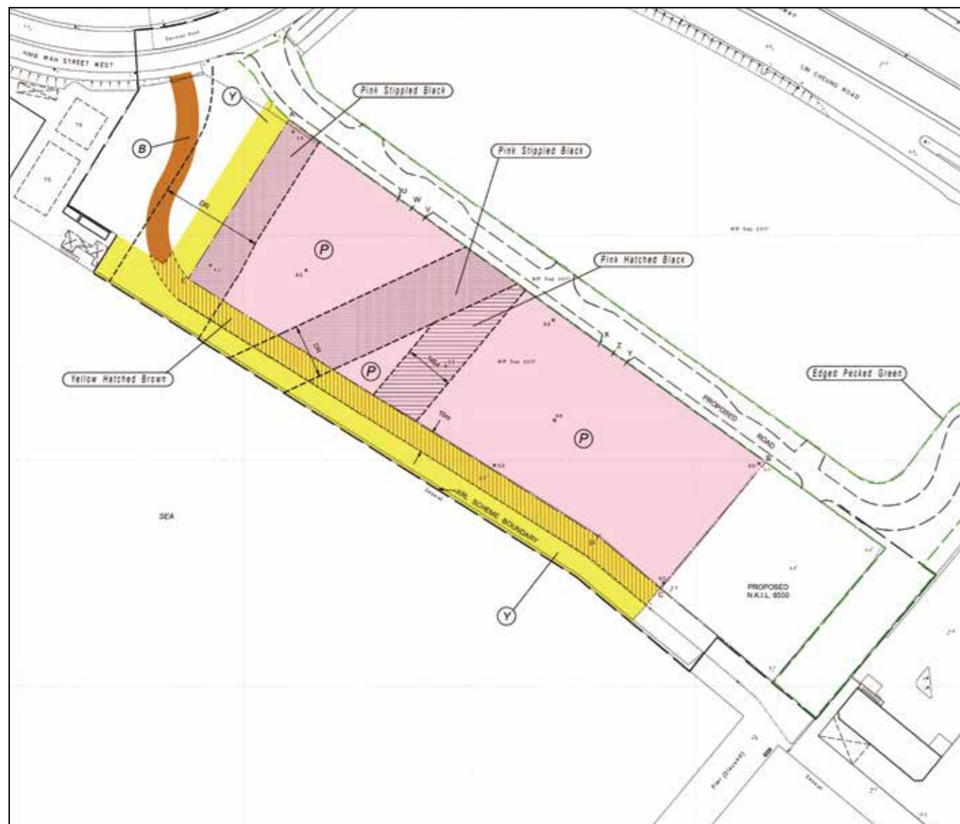
"Plan Showing the Location of the Promenade Area and Drainage Reserve Areas" 「海濱廣場範圍及渠務專用範圍位置圖」
